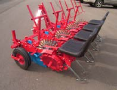
4-rowed type C with 24 gripper planting wheels
